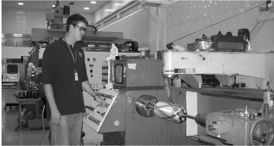
Figure 2.5: Entec filament winding system at the NASA-MSFC facility
